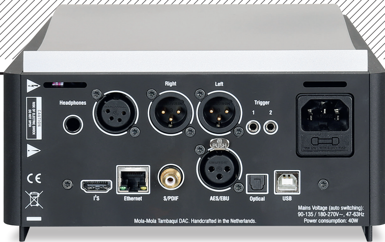
ABOVE: Toslink optical, coaxial and AES/EBU digital ins (to 192kHz/24-bit) are joined by HDMI (iS) plus USB-B and Ethernet (384kHz/32-bit and DSD512). Balanced (XLR) and single-ended (6.3mm) headphone outs are joined by balanced line outs (XLR)
